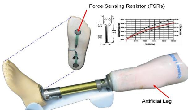
Figure 2. Force sensing resistors on artificial leg
