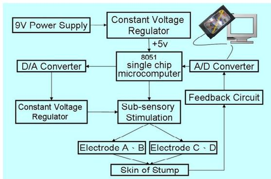
Figure 3. Control signal diagram in subsensory stimulation unit
