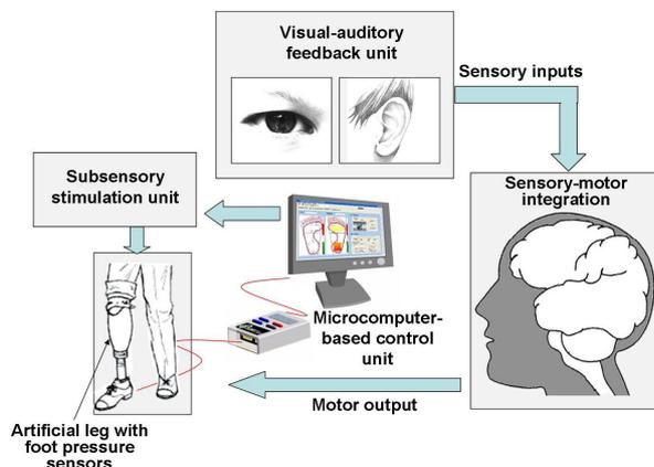
Figure 1. Conceptual design of the proposed sensory feedback system
