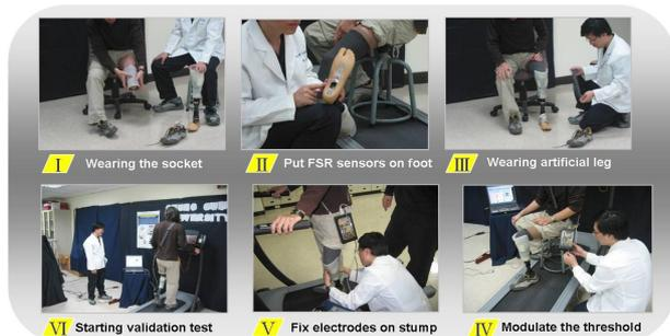
Figure 4. Procedures for dynamic walking stability test
